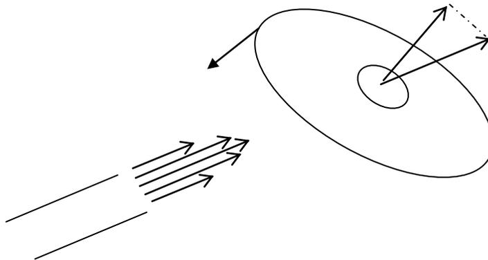
Figure 5a.2 Non-uniform and oblique flow across a moving system boundary.
