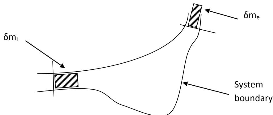
Figure 5a.1 Schematic of a system for analysis of the continuity equation.
