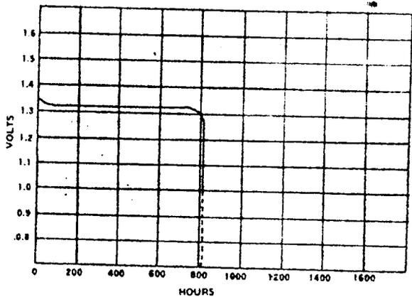
Fig. 1. This is a typical discharge curve of voltage vs time for the Mallory W2 battery for electric watches. The current in this standard test is  $104 \mu\text{A}$  into a  $13\,000 \Omega$  load at  $21^\circ \text{C}$  ( $70^\circ \text{F}$ ). In normal use in a watch this battery supplies a current of approximately  $10 \mu\text{A}$  for a year.
